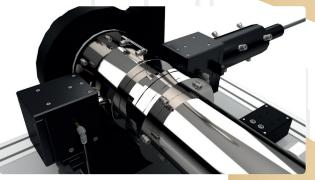
Helium Neon laser, class 2, 2 receiver diodes, neutral density filters (optical density 0,3 and 0,8), air purging
