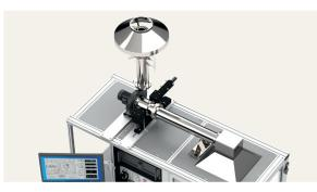
Stainless steel, inner diameter 110 mm, wall thickness 2 mm Centrifugal exhaust fan, power consumption approx. 90 W, heat-resistant up to 300 °C at 2800 rpm and 200 °C at 1400 rpm Electronically continuously adjustable Connector DN 200
